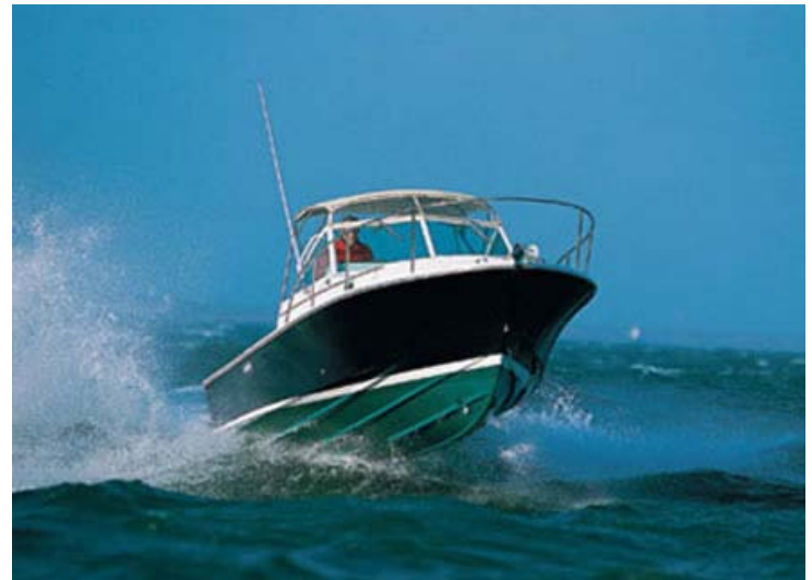
The Hunt Yachts Surfhunter 25 , shown above, along with all models in the Hunt Yachts fleet , are designed by C. Raymond Hunt Associates to take advantage of the deep-V hull form.
