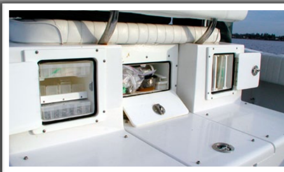
Storage compartments in the back of the leaning post were designed for plastic tackle trays.
